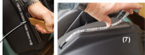
Securing & protecting LED wires under the fender is easier before the fender is installed.
